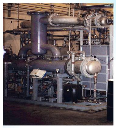
Vacuum evaporation system for the recovery of nitric acid, sulfuric acid and molybdenum. Produces 50-60wt% nitric acid. Evaporator fabricated using 304L stainless steel with zirconium tube bundle, NEMA 4X electrical components, and PLC automation with PC interface.
