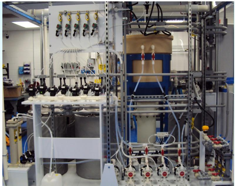
The picture below shows a pilot acid distillation system. The materials of construction are glass components with tantalum heat exchangers assembled with PTFE gaskets. This 10 gallon per hour automated system can be used for the concentration and distillation of various spent or waste acid solutions.
