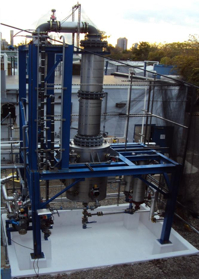
*Mixed acid fractionation system that produces a high purity acid distillation of one acid component using a thermal circulating evaporator with fractionation column.*
